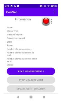
Because the mobile device is not yet connected to the logger, the information fields are initially empty. At this point, it is best to find the optimal position to establish an NFC connection with the logger. NFC works over a short distance (typically just a few centimeters), so ensuring a stable connection is crucial for proper application functionality.
