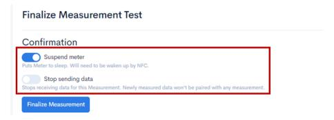
Suspend meter puts the logger into standby mode. The logger would need to be activated via the NFC mobile application when starting the new measurement.
