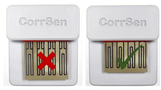
For the CorrSen-D logger, plug the connector into the logger as shown in the picture.
