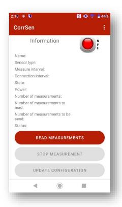
Because the mobile device is not yet connected to the logger, the information fields are initially empty. At this point, it is best to find the optimal position to establish an NFC connection with the logger. NFC works over a short distance (typically just a few centimetres), so ensuring a stable connection is crucial for proper application functionality.
