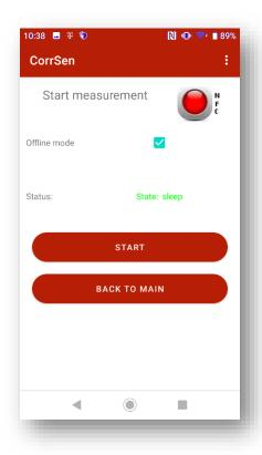
Successful activation is confirmed on the application screen. The logger will switch to measure mode and start recording data. You can verify this by returning to the main menu and checking the Status field – must show the *measure* value.
