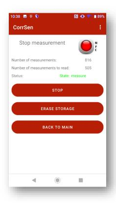
Successful operation is confirmed on the app screen, and the logger switches to the idle state.
