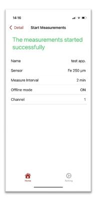
You can verify that the operation was performed correctly by returning to the home screen and reading the logger status – the *Measuring* item must be in the *on* state.
