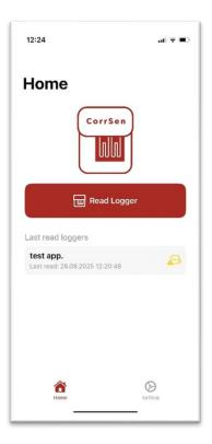
From the Home screen, you can view information about the latest reading sessions from assigned loggers (Last read loggers) or initiate communication with a logger (Read Logger). By tapping on items in Last read loggers, an information window is displayed with details of the latest reading sessions of assigned loggers. The content is identical to the Detail menu described below.
