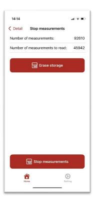
The execution of the function is confirmed on the application screen and the logger switches to idle mode, where data measurement is suspended. At the same time, we can use the **Erase storage** function to delete all measured data (Caution! Before deleting, it is necessary to read the data, if it is meaningful, to the server; the Erase storage function permanently deletes the data from the logger).
