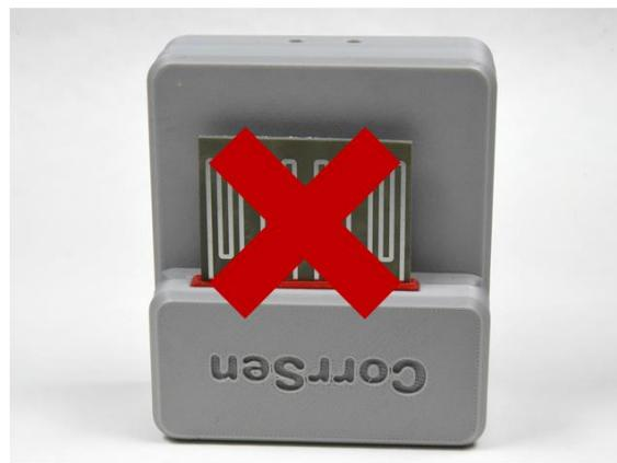
**Caution:** Ensure that the logger is not exposed to the risk of mechanical damage. CorrSen-B loggers must not be exposed to harsh indoor conditions (direct access to water or chemicals) or outdoor conditions.
