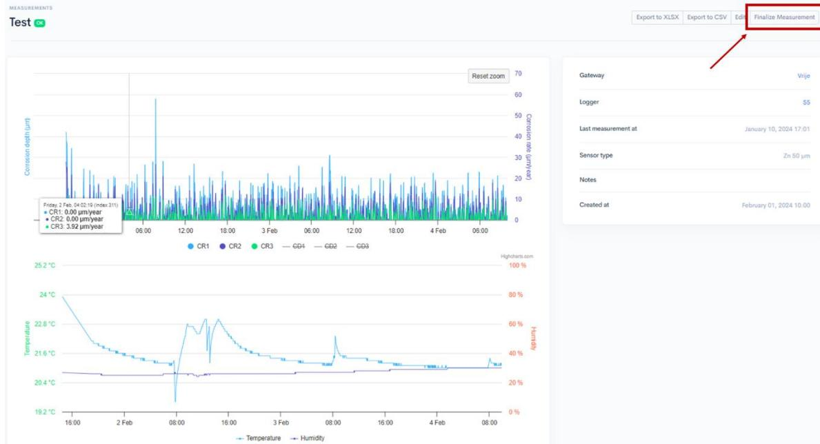
Confirm finalizing the measurement by pressing the *Suspend meter* and *Stop sending data* buttons.
