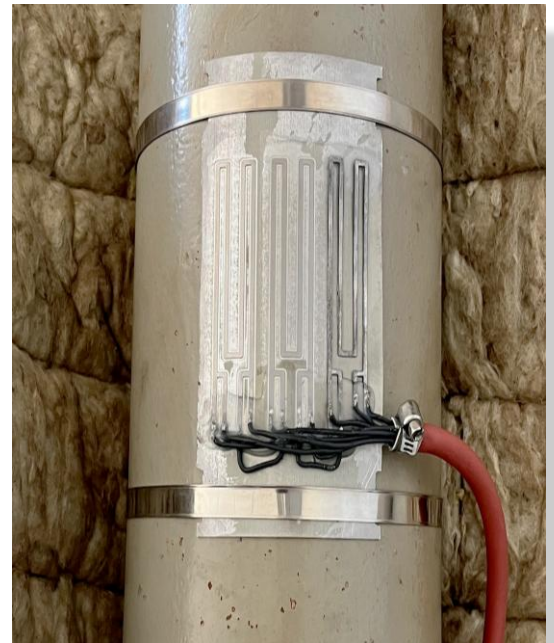
Flexible ER sensor developed for CUI monitoring
